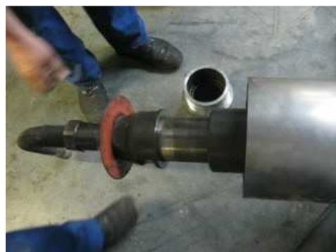
5. Put the End Nut/Tool for Inserting PE/PVC pipes onto the Controller
