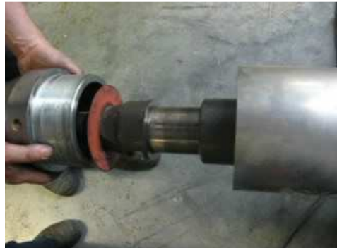
5. Put the End Nut/Tool for Inserting PE/PVC pipes onto the Controller
